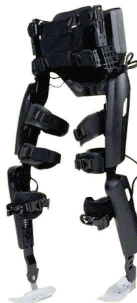
Rewalk Personal 6.0 for rehabilitation of patients suffering lower limb injuries
